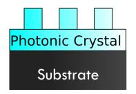
ARC based on planar layers (Bilayer) Nanostructured ARC (Single layer, can be same material than substrate)
