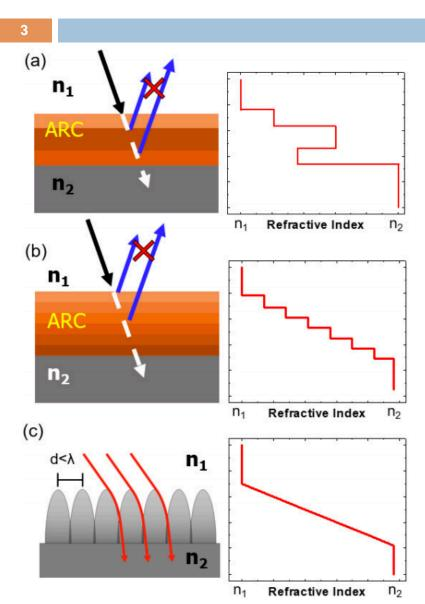
(a) Traditional (and commercial) ARC relies on destructive interference from dissimilar dielectric thin films (typically  $\lambda/4$  thick. These interference-based ARCs are extremely effective in reducing surface reflections at specific wavelengths (e.g. R < 0.01%), but bandwidth and angular response are typically poor.
