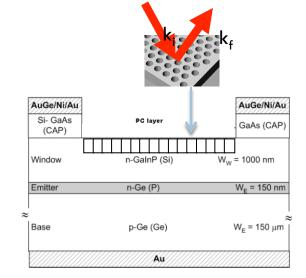
We have used a 2DPC ARC on the InGaP window layer of a single-junction Ge/InGaP solar cell. No degradation of cell performance has been observed.
